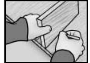
3 Now mark the slots on table leg 1 and the tabletop support. Tip: After marking the length of the slot along its outside edge, mark the width (3/4 inch) by setting one of the cleats on edge and using its thickness as a guide, as shown below right. When you cut out the slots, try to stay directly on the pencil lines so the openings won't be too tight or too loose. You can also drill a 3/8-inch hole at the deepest point of each slot to make it easier to turn the blade and clean out the corners.
