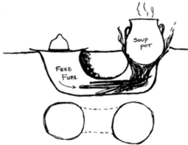
The extreme version of this requires two holes dug about a foot deep and a foot apart. They are connected at the bottom by a tunnel. A pot or grill (or big piece of meat) can be placed over one hole, while the other provides access for fuel and air. The Dakota fire is also very efficient, requiring less fuel, as almost all the heat is put to work. Moderately windy conditions can be handled with a wind screen of rocks or logs.
