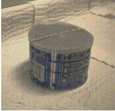
The lid from the coffee can won't fit snug without the original lip of the can so a rubber band is use to keep it together. The stove alone weighed about 0.5 ounces, the stove and pot stand together weighed about 2.5 ounces. The glove and fuel are extra. We were able to bring 2 cups of cold tap water to a boil in about 6 – 7 minutes.
