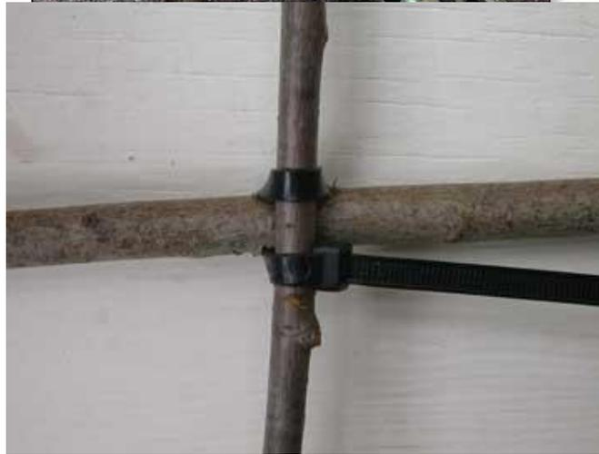
You might also try nylon cable ties. Make sure if you do that you keep the tail of the tie long or if you cut it that you have the sharp cut end facing in away from the cover. You will also want to tighten it so that the gripper part of the tie is inward; since it it faces outward it could cause a hole to wear in your boats cover.
