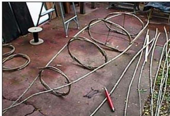
Here you can see ribs joined to the side stringers. Note cords on the two mid-stringers making the bottom of the boat flat. If not flat, the boat tips over too easily.
