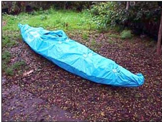
A blue tarp, 12' by 9', was used to cover the frame. You could cover your frame with animal skins if you have them. The tarp was gathered along the top of the boat and fastened together with six [Grip Clips](http://www.gripclips.com). You can also use the rock and cord technique where you place a 1.5" rock under the two tarp layer and then squeeze the tapes into a narrow neck around the rock and tie this tight with a cord.
