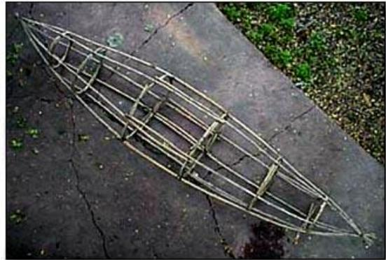
Completed frame. Length is 11.5'. Stringers are about 15' long and overlap the two center ribs. The center ribs are 27" wide and 16" deep. The next out from the center ribs are 19" by 14". The smallest ribs are 13" circles. Spacing of the ribs is 17", 17", 24", 24", 17", 17".
