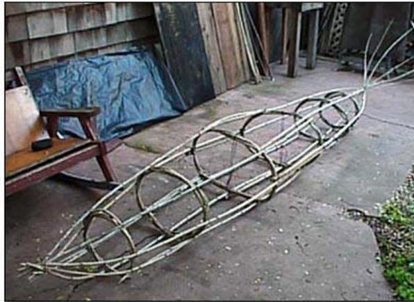
The amount of willow used to make the kayak. If you plan to build this kayak consider building a model. Making a model first of thin willow will make it easier to build a full size kayak. Waxed cord grips the willow and speed along the process. How about a two person boat?
