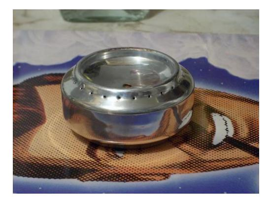
While I was experimenting with early prototypes, it became evident that I wanted a <u>pressure stove</u>. Pressure stoves are more fuel efficient and they have fewer internal parts. I wanted something easy to build but most of all, I wanted a method that would yield consistent stoves. After learning the hard way, I decided that safety was to take precedence over those two requirements. Building a Hannah Stove will take you only one hour. Lets get started with the requirements.
