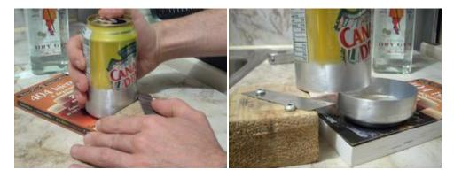
Once you have cut the two cans, it's time to assemble your stove. The Hannah Stove is press fit. If you have peace of mind, you can just align the can bottoms and fit one right into the other. It is
