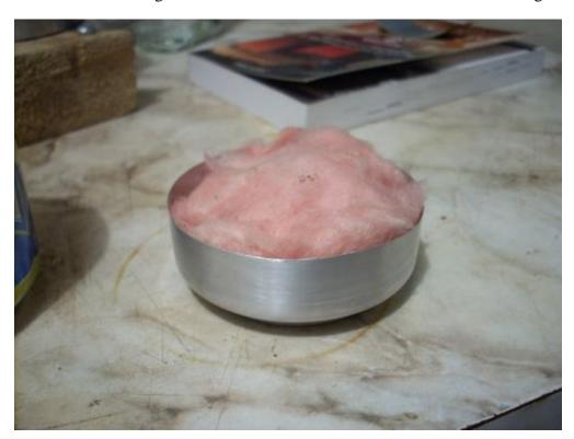
Before you lower the top of your stove over the bottom, drill the filling hole. If you don't, the air pressure might disassemble your stove before you are done, which is really frustrating. Start with 3mm, you can always enlarge later.
